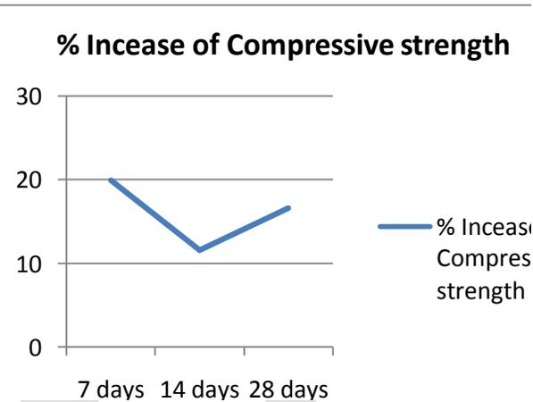
**Figure 3: % Increase in Compressive strength of Auto repairing concrete with ages**
