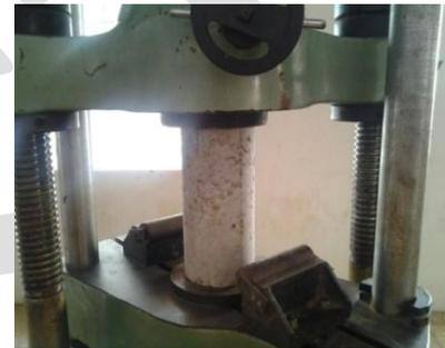
Fig. 9 Cylinder Compressive test
