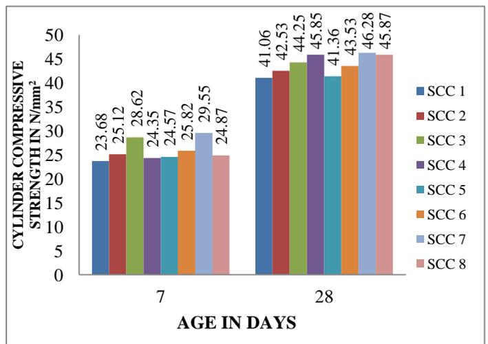
Fig 10 Comparison of Cylinder Compressive Strength at 7 days and 28 days
