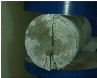
Fig.7. Test setup for Split Tensile Strength
