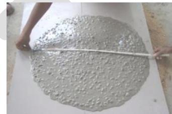
Fig.1. Slump flow test
