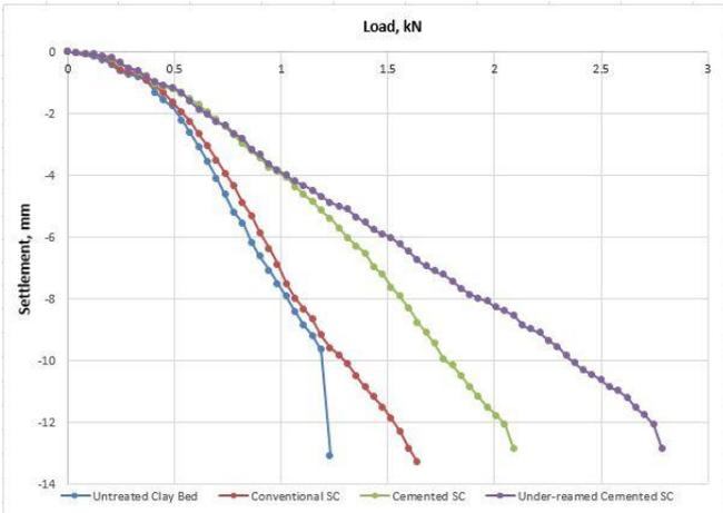
**Fig.1 Comparison of Load vs Settlement curves of untreated clay bed, cemented stone column, conventional stone column and under-reamed cemented stone column**
