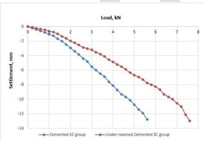
**Fig.2 Comparison of Load vs Settlement curves of cemented stone column group and under-reamed cemented stone column group**
